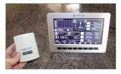
The WeatherRanger comes with an indoor sensor and colour screen
