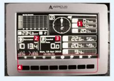
Once everything is in place, connect the display console to the mains and wait for it to synchronise with the indoor and outdoor transmitters. The screen shows weather information including wind speed, 1 pressure 2 and rainfall. 5 Use the buttons underneath 4 to change the settings.
